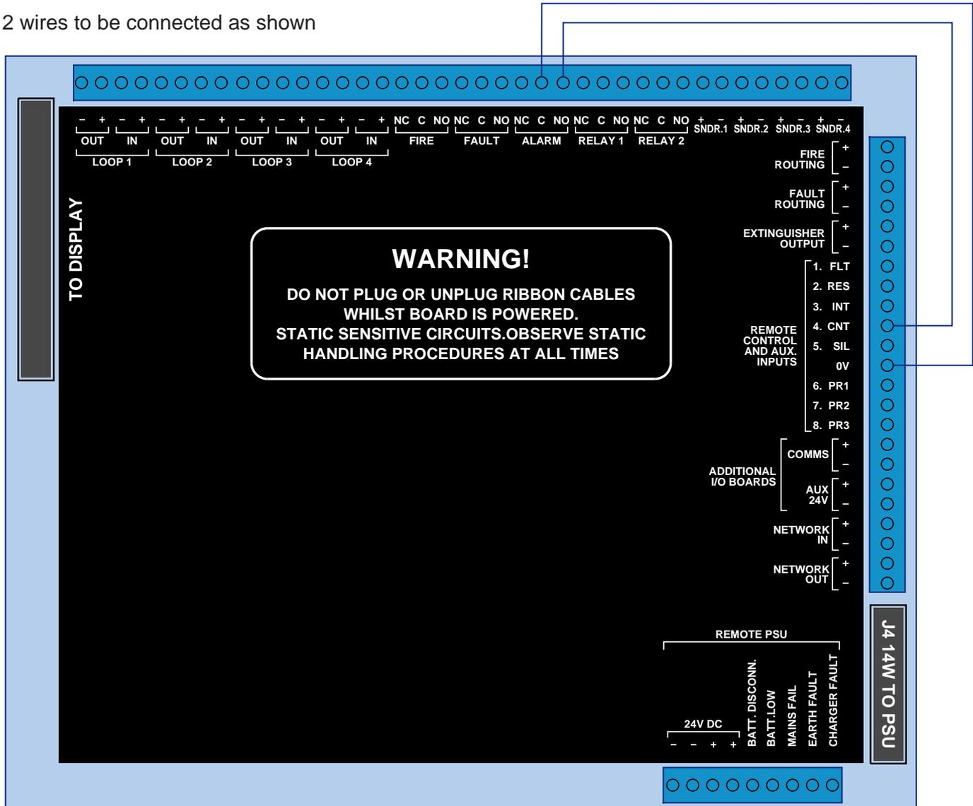
Fig 1 - Panel hardware connections
