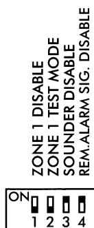
One zone Hydrosense Normal switch positions
